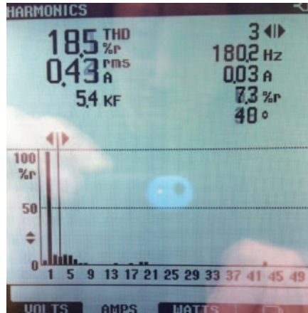
Figure 12 – Powering the same non-PFC 1200 W HMI by means of a transformer instead virtually eliminates the third harmonic current circulating between the two generators.
