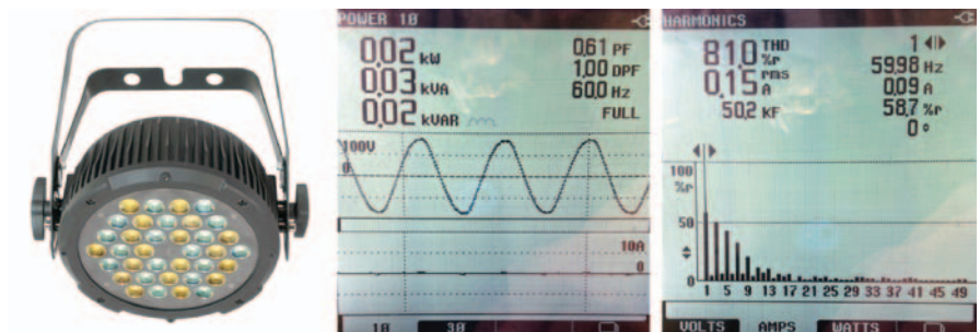
Figure 6 – The Chauvet Slim Par Pro RGB has a PF of 0.61 and total harmonic distortion of 81%.
