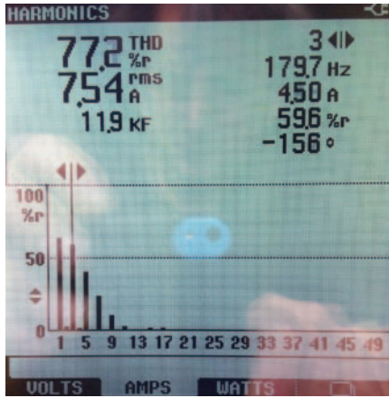
Figure 11 – The harmonic spectrum of a non-PFC 1.2 kW HMI operating on a Honda EU6500 through a splitter box.
