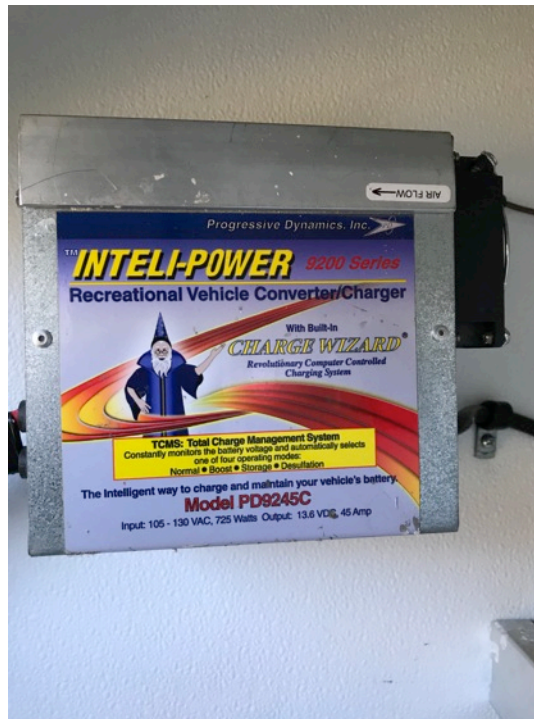
Figure 10: The source of the harmonics drawn by the Flush trailer, a 750W non-power factor corrected switch mode battery charger
