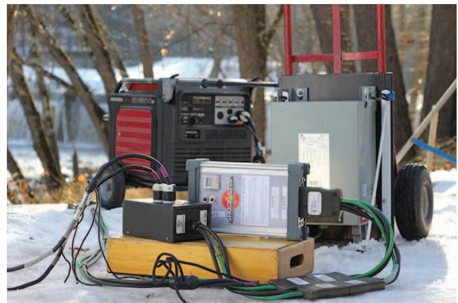
Figure 4 – 60 A Shock Stop Ground-Fault Protection Device with 15 mA trip threshold provides blanket coverage to 120 V distribution system on the secondary side of a 240 V-to-120 V step-down transformer/distro.
